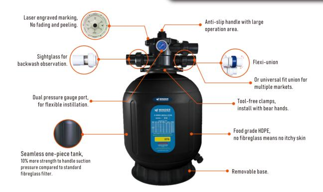
Minder's X series is manufactured using one-piece blow-moulded technology. Greener and safer for you and your pool water.
